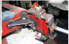
Example of Fully Adjustable Front End with Rose Joints
