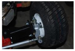
Rear Axle with Drive Gear and Sprocket mounted Inboard Restricts how low your seat can be and should only be done as a last resort
