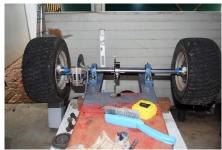
Highly Recommended for lower Seat levels and Centre of Gravity Rear Axle with Outboard Drive Gear, Sprocket and Brake Disc.
